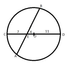
In figure AE\*BE=CE\*DE ( The intersecting chords theorem)
